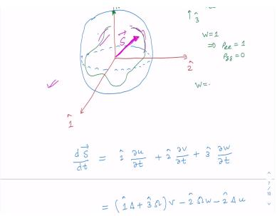
And now I can define the vector this is called the bloch vector and that has a component along this one direction one cap and then say I have this two and three and I can represent it in a diagram soon in the so-called bloch sphere. So, that is what I am going to do now. These vectors it is one cap two cap and three cap these are unit vectors and they are mutually orthogonal to each other in a ficticious three dimensional space.
