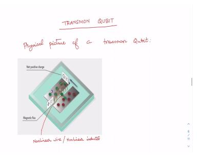
Then finally we discussed in somewhat details about the transmon qubit physically speaking a physical picture was given we discussed about it that it basically consists of 2 metal plates metal plate one and say metal plate 2 connected by a non-linear wire or a non-linear inductance and to discuss it we briefly revised what we learned about the linear quantum linear LC harmonic oscillator.
