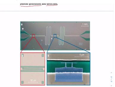
So, this is a very important work and the experimental real transmission line resonator and the cooper pair box is actually shown in this diagram I would not go into the details actually what you see here it is the input end of the transmission line resonator and this is the output end here and in middle here this cooper pair box is placed. I would like to encourage interested people to read the article for experimental details and fabrication.
