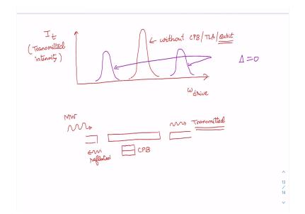
So, far now what the group observed was the intensity of the transmitted beam they plotted the intensity of the transmitted beam as a function of the drive frequency. So, in the y-axis they plotted the transmitted intensity of the signal or the beam here the transmitted intensity and it was plotted as a function of the frequency of the weak oscillating microwave drive.
