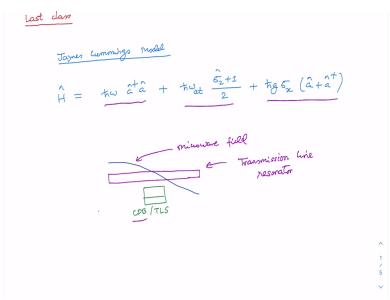
In the previous lecture we started discussing the famous Jaynes Cummings model which described the interaction between a field mode and a 2 level atom or system. In our case the field mode is a microwave field in a transmission line resonator. So, we have a microwave field in a transmission line resonator. On the other hand the atom the 2 level atom is nothing but a cooper pair box.
