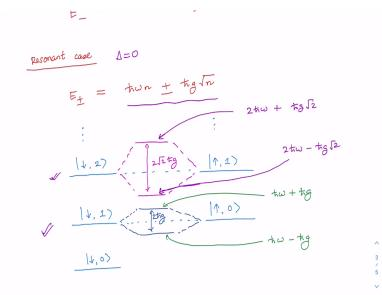
This neutral atom is can be modeled as a 2 level system and this interacts with an optical field. So, this is our optical field one optical field mode inside the cavity and this is our 2 level atom or system and this can also be described using the Jaynes Cummings model and in fact this is the domain of cavity quantum electrodynamics. And what we are discussing in this particular model is actually circuit quantum electrodynamics.
