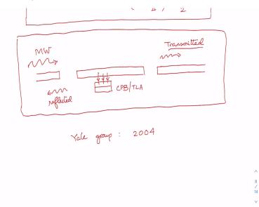
We have a we have a transmission line resonator we know how to get a transmission line resonator. Suppose we have a transmission line infinite transmission line then we break it at 2 locations and then we get a transmission line resonator and then we have a cooper pair box or a 2 level system which is getting coupled to the transmission line resonator at some location.
