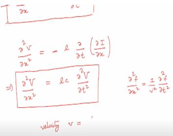
Therefore, I write it as minus and another minus is here so, it would be plus l c delta V del t 2. So, this is the equation for voltage. So, I get del 2 V del x 2. Actually, it is pretty easy to see if you compare this equation with the classical wave equation that is your del 2 f del x 2 = 1 / v square del 2 f del t 2. From a classical wave equation the velocity so this is, do not get confused with this V.
