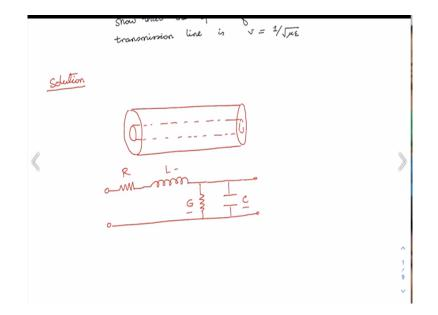
So, you have an inner conductor and you have an outer conductor. So, you have said we have a coaxial cable like this. This is the outer conductor and this is the inner conductor. And this coaxial cable has a circuit representation and in circuit representation it is represented by a resistance in series with this inductor L resistance R and then we have this conductance. In the class, actually, you have taken a very simplified model of the transmission line.
