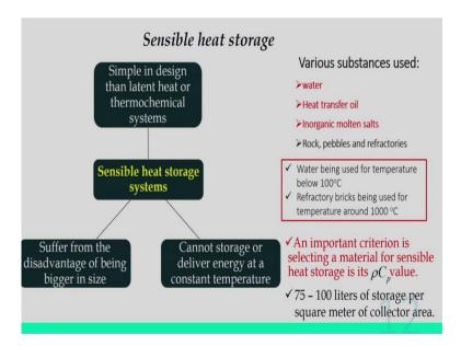
Now, come to the sensible heat storage system, which is simple in design than latent heat or thermal chemical storage system. But it has got some disadvantages, like it requires a bigger size of systems. And it cannot store or deliver energy at constant temperature, that is the major drawback.
