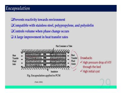
So, encapsulations is done to prevent reactivity towards environment. Then compatible with stainless steel, polypropylene and polyolefin. Controls volume, when phase change occurs, which is very, very important. A large improvement in the heat transfer rates, if we make this kind of arrangement.
