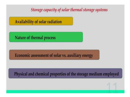
So, this storage capacity of solar thermal storage systems depends on availability of solar radiation, nature of thermal process, economic assessment of solar versus auxiliary energy, then physical and chemical properties of the storage medium, which are going to be employed.
