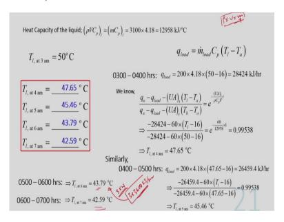
Now here, in this case, the heat capacity of the liquid can be calculated by  $(\rho C p V)_l = (\dot{m} C_p)_l$ , because  $\rho \times V$  is nothing but mass. Since mass is known to us, so that is why,  $\rho \times V = m$  is considered in this problem. So, this m is 3100 multiplied by specific heat is 4.18, so it is comes around 12958 kJ/ $^{\circ}$ C.
