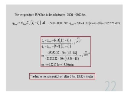
So, the temperature 45  $^{\circ}$ C has to be in between 5 to 6 hours and we need to find out the q<sub>load</sub> by using this expression between 5 to 6 and it is found to be about 25252.22 kJ/hr. So, we can find out the time.
