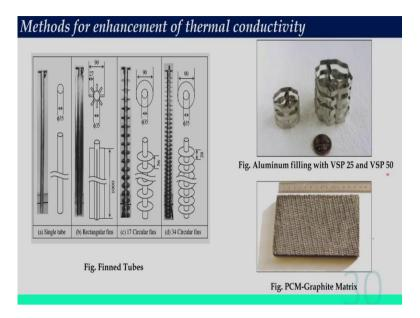
And also, there are different other enhancement method like finned tubes. So, this kind of fin, we can make and we can insert there, to increase the thermal conductivity of the system or maybe effectivity of the PCM system.
