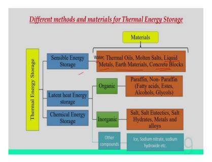
And if we see that the kind of material used for all these thermal energy storage system, we can see what are the different materials can be used for sensible energy storage. We can use variety of material like water, then concrete blocks for solids, and for high temperature application, thermal oils, molten salts, liquid metals, then earth materials.
