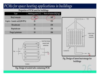
So, this table shows the properties of PCM used for thermal comfort in buildings. So, these are the different types of PCM used for building. Suppose we need to maintain at, say, 20 °C
