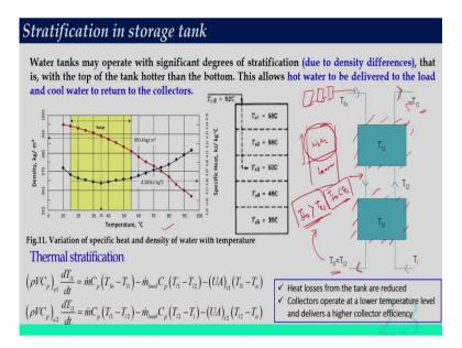
So now, let us consider the case for stratification in storage tank. This water tanks may operate while significant degree of stratification due to the density difference, that is, with the top of the tank hotter than the bottom. This allows hot water to be delivered to the load and cold water to return to the collector.
