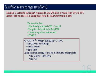
Now, we will discuss one very basic problem, how this sensible heat storage can be calculated. So, calculate the energy required to heat 270 L of water from 15 to 55 °C, assuming that no heat loss is taking place from the tank where water is kept. So, values given are density of water is 993, Cp is 4.18 kJ/kgK, price of the electricity is 6 kWh; then 1 J= 1 Ws. And  $\Delta T = 40$  °C.
