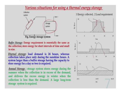
So, so what are different situations for using thermal energy storage? As you can understand now, if you consider this kind of system where one flat plate collector is involved where solar radiation is received and useful heat is generated and that can be stored at a particular time and whenever required that can be utilized.
