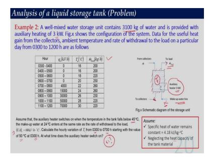
So, this problem goes something like, a well mixed water storage unit, means that  $T_l$ , if you consider is  $T_l$ ,  $T_l$  is constant for 1 hour duration, contains about 3100 kg of water. And is provided with auxiliary heating of 3 kW. So, this 3 kW auxiliary heating is given here. So, figure x shows the configuration of the system. So,  $\dot{m}$  is the mass flow rate from the collector and introduced in the tank.
