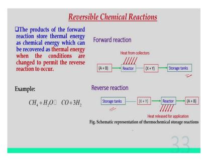
So, the product of forward reaction store thermal energy as chemical energy, which can be recovered as thermal energy when the conditions are changed to permit the reverse reaction to occur. So, already we have discussed the examples and this is the way it reacts.
