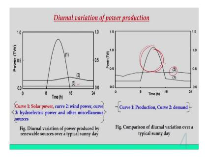
This figure shows the diurnal variation of power production by renewable sources over a typical sunny days. So, this 1 indicate the energy produced by solar energy and then, 2 marked in the curve shows the variation of energy generated by wind power and then 3 in the figure 1, shows about the power generation by hydroelectric power and other miscellaneous sources. So, this is more or less constant.
