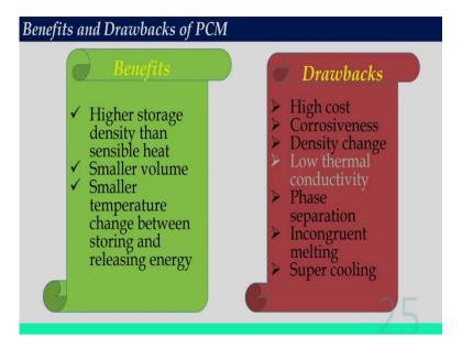
What are the benefits and drawbacks of PCM? So, this benefits includes higher storage density than sensible heat, smaller volume, smaller temperature change between storing and releasing energy. So, drawbacks are high cost, corrosiveness, then density change, low thermal conductivity, phase separation, and incongruent melting, that is not uniform, melting is there, then super cooling; before it reach, the cooling is also taking place.
