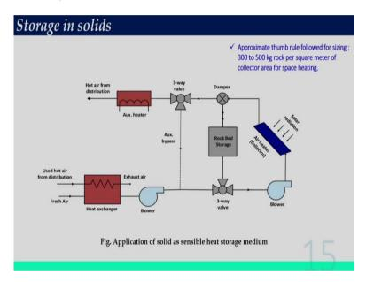
So, this is the case what we are discussing about. So here, this is our solar air heater where air is heated and that can be stored in a rock packed, or rock bed storage, that is a packed bed. And whenever required, that can be used based on the applications.
