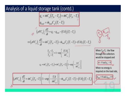
Now again, we can relate this  $q_u$  and  $q_{load}$  with respect to inlet and outlet fluid temperature. So,  $q_u = \dot{m} C_p (T_{fo} - T_{fi}) = \dot{m} C_p (T_{fo} - T_l)$ . And  $q_{load} = \dot{m}_{load} C_p (T_l - T_l)$ . So,  $T_l$  maybe  $T_a$ . So that way, we can relate this  $q_u$  and  $q_{load}$  in terms of inlet and outlet fluid temperature.
