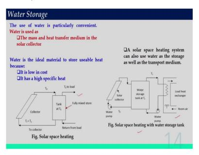
So normally, water is used in most of the cases and this water is used as heat and mass transfer medium in the collector. And also it is used because, it is low in cost and has a high specific heat. So, these are the configurations by which solar energy can be stored in a storage tank and that can be used based on the applications.
