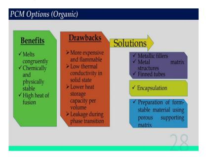
Now, let us pay attention about organic PCM, what are benefits and demerits. So, it melts concurrently, and chemically and physically stable and high heat of fusion in case of organic material. And drawbacks are more expensive and flammable, and low thermal conductivity in solid state. And lower heat storage capacity per volume. And leakage during phase transition. These are some of the drawbacks.
