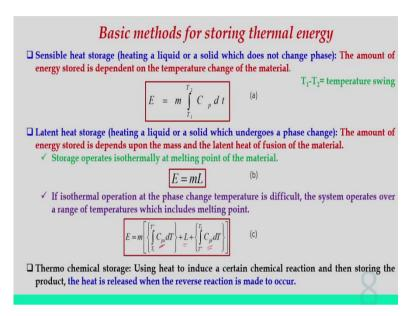
So now, let us study about basic methods for storing thermal energy. So, what are different methods? As you can understand now, so we have sensible heat storage, then we have latent heat storage, and thermochemical storage. So, for sensible heat storage, where there is no phase change occur, only temperature rise will be there. The amount of energy stored is dependent on the temperature change of the material.
