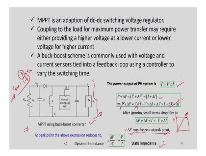
So, this MPPT is adoption of the dc-dc switching voltage regulator. So, coupling to the load for maximum power transfer may require either providing a higher voltage at lower current or lower voltage at higher current. Normally, a buck-boost scheme is commonly
