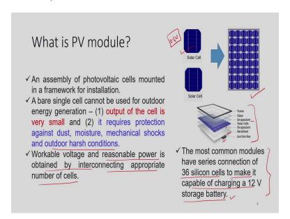
PV module is an assembly of photovoltaic cells mounted in a framework for installation. As you can see, this is a single solar cell, this single solar cell or you can say bare single cell cannot be used for outdoor applications; because its output is very less. As we can say, it will give about 0.6 V. So, single cell will provide about 0.6 V, so this cannot be used for many of the practical applications, if we are proposing for outdoor applications.
