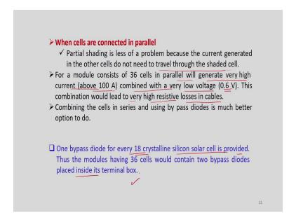
Now, come to the situation, when the cells are connected in parallel. This partial shading is less of a problem because the current generated in the other cells do not need to travel through the shadowed cell. This is one important aspect. And for a module consists of 36 cells in parallel, will generate a very high current above 100 A, and combined with a very low voltage is about 0.6 V.
