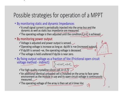
So now, what are the different strategies adopted for operation of an MPPT? So, first one is by monitoring static and dynamic impedances, and second one is by monitoring power output, and third one is by fixing output voltage as a function of open-circuit voltage. This is also known as frictional open-circuit voltage method, and this falls under indirect method.
