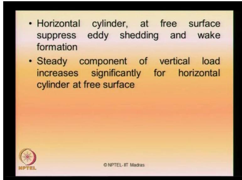
Horizontal cylinders at free surface suppress eddy shedding and the wake formation. Steady component of the vertical load increases significantly for the horizontal cylinder at the free surface. So, as we move towards a free surface horizontal cylinders attract more forces. There is something called blockage factor which is very important in the design which is an important aspect an outcome of a FSI.
