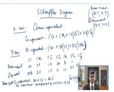
So in the case of Schaeffler diagram so you have x axis as the chrome equivalent and this is also known as chrome equivalent. So that will be basically % chromium + % molybdenum +1.5% silicon + 0.5% columbium. So this is normally the formula for the chrome equivalent. Similarly, you will have the nickel equivalent. Now nickel equivalent is % Nickel + 30% carbon + 0.5% manganese.
