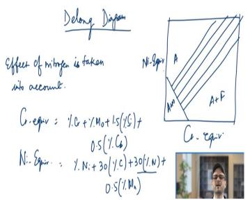
There is another diagram also which is along with Schaeffler diagram used in the case of welding and that diagram is commonly known as Delong diagram. So you will have also so that is not shown here, but that is also similar to the Schaeffler diagram. However, in this case it is normally used you know to take into the account the effect of nitrogen. So here also you will have the nickel equivalent and the chromium equivalent you know on the y axis and the x axis.
