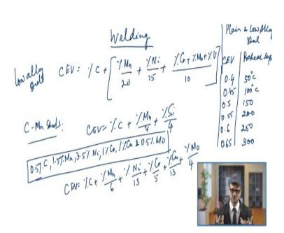
Now in case of welding many a time you may have to go for the pre or post weld heat treatment. So you may have to go for preheating or post weld heat treatment and that depends upon the carbon equivalent value. So if the carbon equivalent value will be more because you know for this stress relieving or so, because there will be chance of cracking. So apart from carbon if you have some other alloying element in that case that will also add too.
