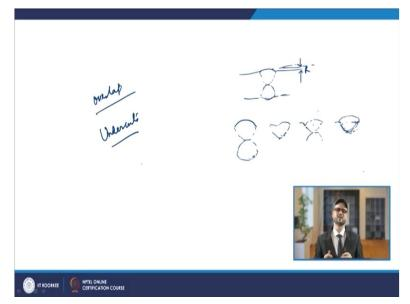
So, if you look at a proper butt weld. So on both these sides you have, so this is how, you know, you will have the convexity. So, this way what is acceptable, butt weld profile should look like. Again, you will have the R, which is here that is defined, this R is basically just denoting the reinforcement. So, and then in butt weld, there may be a different kind of problems like you may have the excessive convexity.
