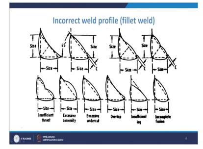
So, if you look at the weld profile, so, normally what you see is that this is the desirable weld profile in the case of fillet welds and this is how you take it as acceptable ones. So, this may be acceptable in those cases. So, if you see that this C is basically showing the convexity, which is shown here and here also. So, this may be, acceptable and what you desire is like this, so, this is what is desired, normally, in the case of fillet weld.
