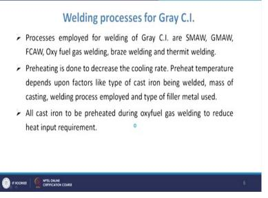
Coming to welding processes for gray cast iron. The processes which are employed for the welding of gray cast iron are shielded metal arc welding, gas metal arc welding, flux-cored arc welding, oxyfuel gas welding, bridge welding, and thermit welding. So, all these
