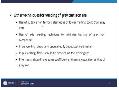
Other techniques for welding of gray cast iron, so that is what we normally do, is that we use suitable non-ferrous electrodes of lower melting point than the gray cast iron. So, that is one way which we do for minimizing the excessive cooling rate. By this process we can do that. We do the use of skip welding technique to minimize heating of gray iron components, as we have understood that we go for skip welding as well as we go for back-step.
