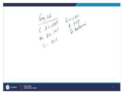
If you talk about the gray cast iron, the typical percentage carbon is about 2.5 to 3.8%, silicon will be 1 to 2.8%, then you have manganese as 0.4 to 1%, phosphorus is 0.15%, sulfur is 0.1%, and iron is balance. What you see is that you have the carbon and silicon are in considerable amount. Anyway (carbon + silicon)/3 is also defined as the carbon equivalent, even phosphorus also is taken into account in that way.
