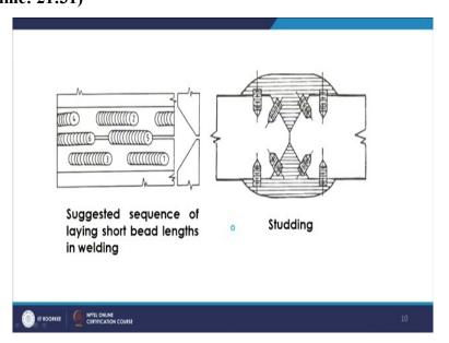
We are doing studding to give quite a good strength in those cases. So, here it is showing the short bead length which is being provided and this is studding way, this is a good way of welding of welding practice.
