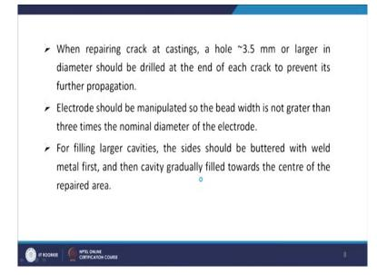
Then, next, when we are repairing the crack or the castings a hole about 3.5 mm or larger in diameter will be drilled at the end of each crack to prevent its further propagation. So, that is another way to avoid the propagation of these crack because in the case of the cast iron there is chance of crack propagation and because they are brittle materials so that way it becomes even more severe.
