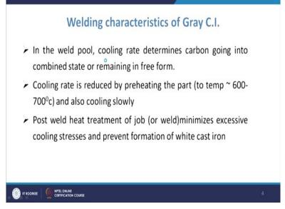
If you see in the weld pool, the cooling rate determines carbon going into the combined state or remaining in free form. So, certainly, as we know that when you are increasing the cooling rate, then most likely you are going to have the carbon going into the combined forms, it will make Fe<sub>3</sub>C and the whole purpose of making the gray cast iron is lost. That is what is happening normally in the case of welding.
