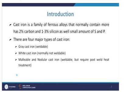
You have the gray cast iron which is weldable and we will talk about its traits later. Then, you have white cast iron which is considered having very poor weldability. Then you have the malleable cast iron and then you have the nodular cast iron. So, you have these four types of cast iron which are available as the types of cast iron. Malleable and nodular cast iron they are weldable, but they require post-weld heat treatment.
