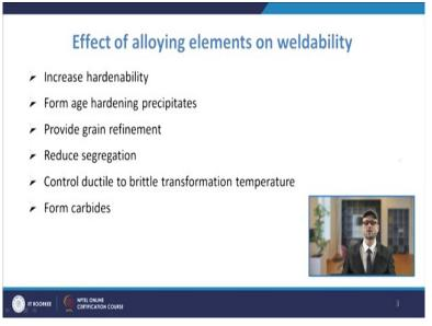
Now, coming to the alloying elements, there are alloying elements which are used in the material. Alloying elements have a say on the weldability of the material. So, the alloying elements have their roles in different ways like the increase the hardenability. Many of the alloying elements which are used they will be increasing the hardenability of the material that can be expressed even in terms of carbon equivalence, that we will see.
