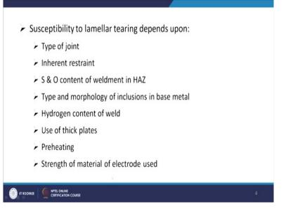
So, if you talk about the susceptibility of the lamellar tearing, the material whether it will be susceptible to the lamellar tearing that will be depending upon the, one is the type of joint, second is the inherent restrain that is there. Then, you have the sulphur and oxygen content of weldment in the head affected zone. Then, type and morphology of inclusions in the base metal. You have the hydrogen content of the weld and the use of thick plates.
