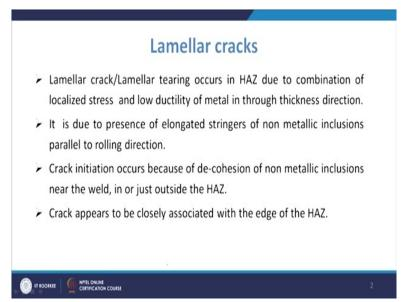
So, lamellar crack or lamellar tearing that is occurring in the HAZ due to combination of localized stress and low ductility of metal through thickness direction. So, basically, in that through thickness direction these tearings are observed and it is because of the combination of the localized stress as well as the low ductility of the metal.
