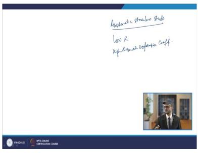
Now, in the case of the austenitic stainless steels, if you look at the stress corrosion cracking of the austenitic stainless steel, so in austenitic stainless steels for these materials you have low thermal conductivity and you have high thermal expansion coefficient. So, you have low K and high thermal expansion coefficient. So, what is happening is that when they are limiting they are subjected to the chloride containing corrosive media.
