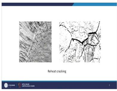
So, this is basically the example of these reheat cracks which you can see here. This is how the reheat crack looks like. So, if you try to avoid these formation of reheat cracks, there are certain steps by which you can avoid these reheat cracks and these are that you should have the eliminate vanadium content in the thick sections and then you can have the design to have the minimum restraint, and further, you can have higher preheat temperature.
