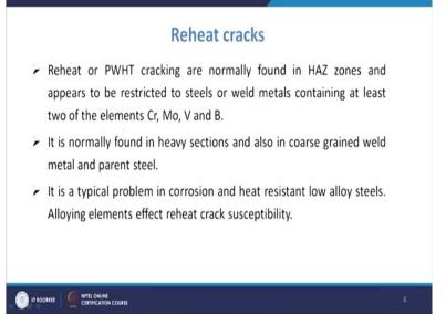
So, reheat or the post weld head treatment cracking are normally found in HAZ zones and appear to be restricted to steels or weld matters containing at least two of the elements, chromium, molybdenum, vanadium, and boron. Normally, if any of these two elements are there in the steel, so they are more likely to have the chances of having the reheat cracks. So, if you look at these elements, they are basically the strong carbide formers.
