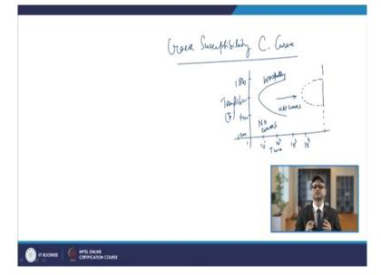
So, if you see, for materials like Waspalloy or Inconel, so what has been seen is that, so this will be temperature and this will be time, so this is on the log scale, so it will be 10 1, 10 2, 10 3, so what is seen is that this curve is found and in that case you have no cracks on this side. So, this is your crack susceptibility C curve, how much it will be susceptible to the crack and this is for Waspalloy. And if you go for alloy 718, for alloy 718 it goes like this.
