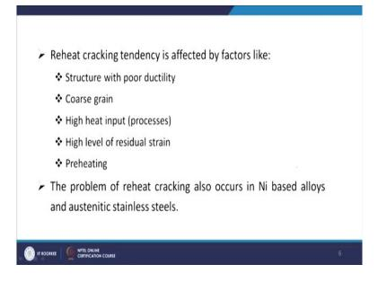
Then, you have high heat input processes, whichever has the specific high heat input processes are there like electroslag welding or submerged arc welding processes, the joints which are made by these processes they are more susceptible to reheat cracking of the specimen. Also, many a times it is affected by the section size also. So, many a times it is more for the higher thick sections, more than, say, 50 mm section thicknesses.
