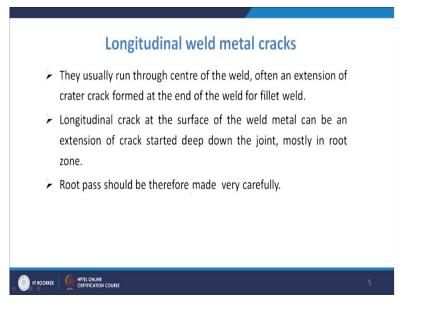
Now, the longitudinal weld metal crack, they usually run through the center of the weld, often an extension of the crater crack form at the end of the weld for fillet weld.
