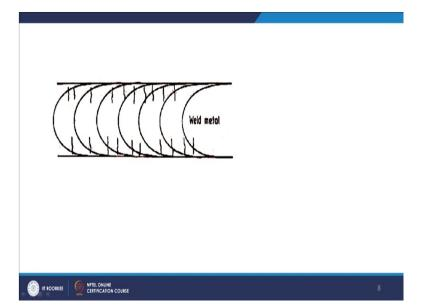
So, these cracks will be normally running so, they are across this or perpendicular to the weld axis their movement is.
