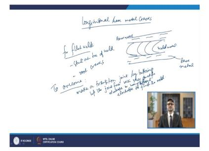
So, as you have seen that you have longitudinal weld metal cracks that will be in the weld bead, but, in these cases, these longitudinal base metal cracks, so they will be parallelly running to the weld and they will lie in the base metal basically. So, what is happening, so, there they will appear like so, if suppose, you have the weld bead appearing like this and this side you are base metal is there and this is your weld metal and this side is base metal.
