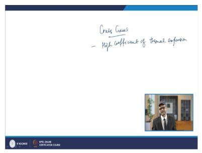
So, normally when you are welding any material which has very high coefficient of thermal expansion like austenitic steel, so, in those cases, your crater cracks are very likely to be found.
