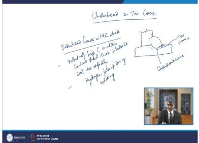
Then depending upon the location of the cracks, you have another category of the crack that is your underbead and toe cracks. So, these cracks **so**, they are the surface cracks in the base metal and they are under or near the weld. So, when they are, the surface cracks in the base metal under or near the weld, so that is known as the underbead cracks. So, we had seen yesterday this is your weld bead looks like and you have fillet weld, typical fillet weld will be shown like this.
