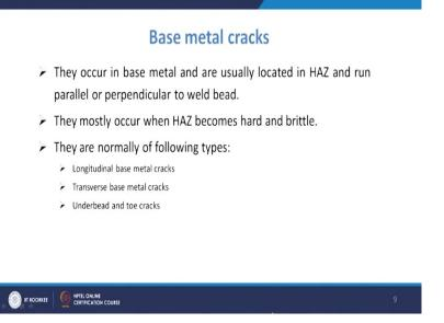
And that may be because of many reasons and so you have the existence of these different types of base metal cracks and they are of different categories like you have the longitudinal base metal cracks, you have transverse base metal cracks, you have the underbead or toe cracks, that is what normally is because of the positions where they are occurring. So, if you talk about the longitudinal base metal cracks.
