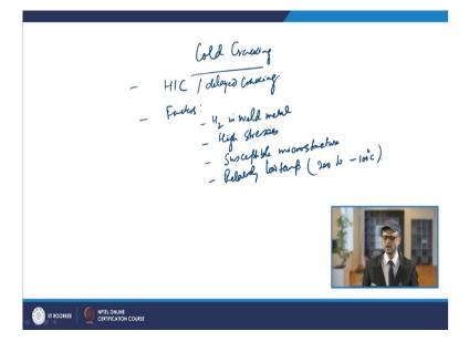
So, as we had the studied that the cold cracking is also known as the HIC or hydrogen induced cracking and it is also known as the delayed cracking. So, it occurs late, so it is known as the delayed cracking and normally you have the welding of high strength steels then these cracks are developed. And the factors which are present simultaneously which are responsible for these type of cold cracking are the hydrogen in weld metal, then you have the high stresses.
