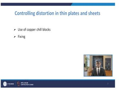
So, you know, you have the copper tubes braced to the copper holding clamps and then water is circulated through that, tubes, so, during the welding. So, that way, if that basically decreases the temperature in those cases, it is likely that your distortion will be smaller. Then you have some other way also, to reduce the distortion in the case of plates and one is the method of fixing. So, you try to have the frame as rigidly as possible to avoid the bending and angular distortion.
