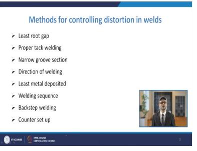
So, these are the methods, which are used for the control of, distortion in the welds. Now, these methods include the least root gap as we see, you have proper tack welding, you have narrow groove section, direction of welding, least metal deposited, welding sequence, backstep wielding, counter set up. So, all these methods are the ones, which should be, followed, which these should be practiced to ensure that there is a minimum amount of distortion that is taking place.
