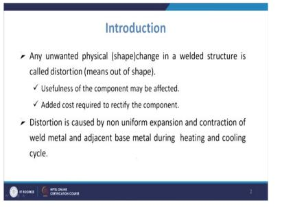
As we know, that distortion means any unwanted physical shape change in a welded structure, that is called distortion. Distortion means it is becoming out of shape, so no longer you can use them. So, basically, if the structure is distorted, its usefulness will be affected. You cannot have the same value of that component as it has been if it would have been undistorted or it would have been in a proper shape.
