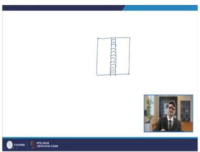
If we talk about the different types of distortion in welding, if you talk about a particular weld, what happens is that, suppose you have a butt weld which is going on, if suppose this is the bead, this is your weld bead which is there on this seat, so what happens is that there may be distortion in different way on this specimen and that will be mainly in terms of shrinkage or in terms of the angular distortions or it may be bowing or it may be twisting.
