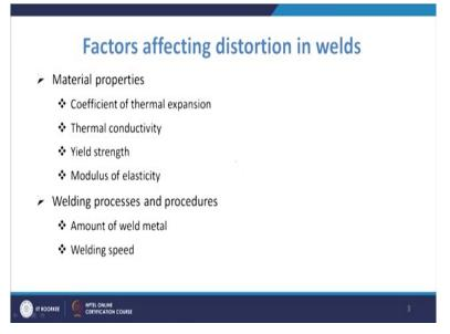
So, coming to the effect of or the factors which are affecting the distortion in the welds, so you have certain parameters which basically affect the distortion in the welds, and among those factors you have the material property. So, there are different material properties and each of the material property may have a positive or negative contribution towards the distortion which is caused in the welded specimen.
