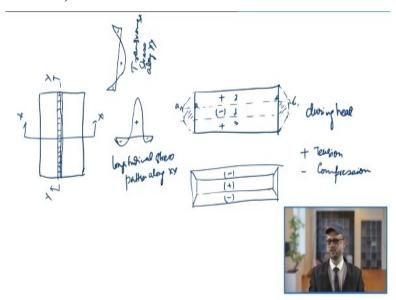
Say you have this way a steel plate and it has 3 zones. So basically we talk about these 3 zones in this steel plate. Now what happens that if suppose we take this as you know 1, 2 and 3, so if suppose it is subjected to heating. So we will talk about the internal stresses which are developed in this plate and what happens that you know as the zone 1. So this is your zone 1, zone 2 and zone 3.
