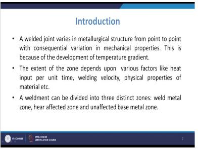
Now, extent of this zone will be depending upon various factors like heat input per unit time, then you have the welding velocity and you have the physical properties of the material like the thermal conductivity you know or thermal diffusivity in true sense you can say, then you have the melting point. So, all these things are also determining that what will be the you know width of or the dimension of that particular zone will be.
