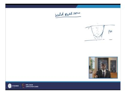
So, coming to you know weld metal zone, so if you talk about you know the weld metal zone, so weld metal zone is basically you know formed by the solidification of the weld pool. So, you know you will have the melting you know, in the central part you will have melting of the original material as well as you have the melting of you know filler metal. So, they are getting melted and that is why it is known as the weld metal zone you know zone.
