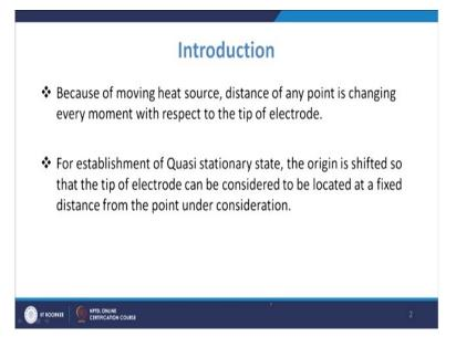
So distance of any point as it is changing with respect to the tip of electrode and for establishment of Quasi stationary state what we do is originally shifted, so that the tip of electrode can be considered to be located at a fixed distance from the point under consideration. So that way you are changing that and what we saw in our you know earlier lecture.
