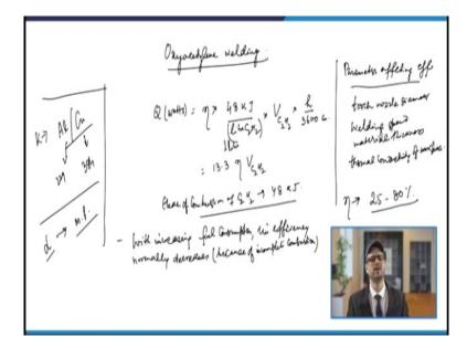
So, suppose you know you should take the oxy acetylene welding, so as we know that the heat is transferred by the combustion of the oxy fuel and the fuel which is normally hydrocarbon fuel that is ignited and the heat which is released from there that goes and heats the region where the welding has to take place. So, in those cases your Q that if you are measuring this in terms of watts, so it will be you know,  $\eta$ .
