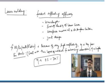
Next you know we will talk about the laser welding now, as we know that in the laser we will use the lasers and in the case of laser welding basically, the efficiency will be affected very much because of the wavelength and the energy density of the laser beam, so here the factors which are affecting the efficiency, so it will be say the wavelength, then you have energy density of the laser beam, you have a work piece material and its surface condition and joint design.
