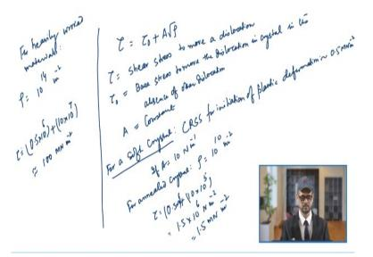
It is found to vary with the square root of the dislocation and keeping the constants we write it like  $\tau_0 + A\sqrt{\rho}$ . So basically what happens that this  $\tau$ ,  $\tau$  is the shear stress to move a dislocation and you know this  $\tau_0$ this is basically the base stress to move the dislocation in crystal when there is no other dislocation. So in the absence of other dislocation.
