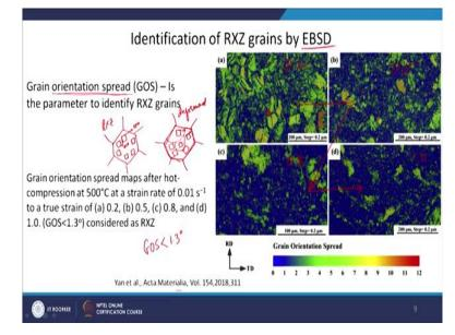
Now, there is another very important characterization technique, is electron backscatter diffraction EBSD and why I was taking that here is because this is one of the very important technique now, to characterise the recrystallization process in the material. And as I told you that in this particular technique, actually you find out the orientation of each grain. So, basically orientation of the unit cell that how the unit cell is oriented in different grains.
