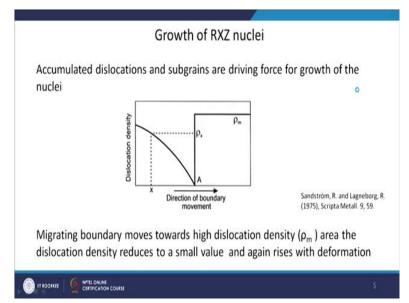
Now, growth of recrystallization nuclei if you see the growth schematic diagram is there (refer to above figure). So, at A is your the newly formed recrystallized grain, the boundary of that which is growing. So, if you see in terms of dislocation density where this grain boundary is, the dislocation density is very low. Just ahead of this boundary which is moving, you have a dislocation density of the matrix.
