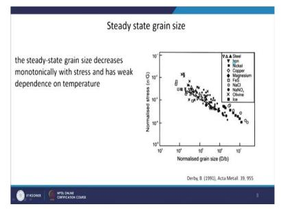
So, of course, it will also affect the grain size of the material. So, if you want to measure the steady state grain size means after the recrystallization the steady state which is taking place. So, a steady state grain size if you measure that decreases monotonically with stress and weak dependence on temperature. So, it is actually strongly dependent on the stress and weak dependent on the temperature.
