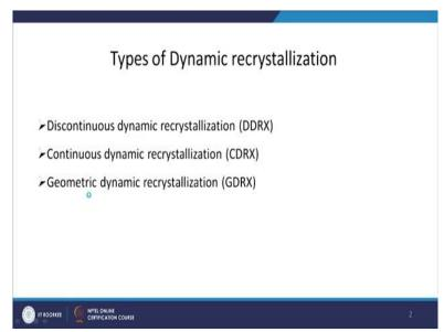
So, basically dynamic recrystallization there can be three types of dynamic recrystallization, which we will be covering one by one. In that discontinuous dynamic recrystallization is the first one which we are going to cover then the next one is continuous dynamic recrystallization and the geometry dynamic recrystallization. Actually most of the studies and the modelling of numerical modelling or analytical modelling is done on the discontinuous dynamic recrystallization.
