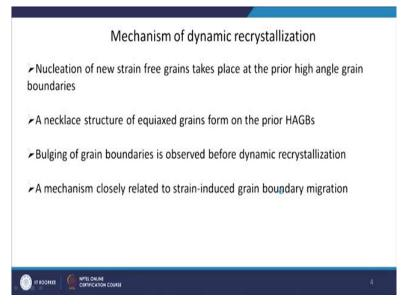
And where it will nucleate or where this will nucleate as in case of phase transformation if you know the new ferrite grains will nucleate at the prior austenite grain boundaries. So, similarly in this case nucleation of new strain free grains will take place at the prior high angle grain boundaries and around that you have dislocation density, so that is where it will start. And because it will start at those boundaries it kind of form what people call it as a necklace structure.
