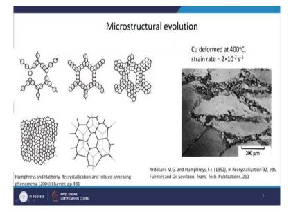
Now, as I told you that microstructural evolution if you see in case of dynamic recrystallization (refer to above figure). So, as I told you the if you take a particular grain. This is the prior grain which was there before the deformation started. And now, as the deformation is progressing you have more dislocation density and also there is a higher dislocation density in general if you see how the dislocation are distributed within the grain.
