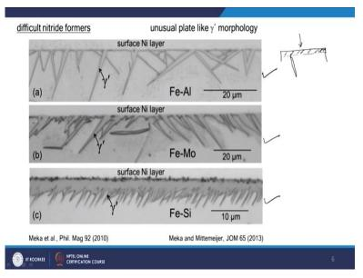
So, what you shown in this slide (refer to above figure) is, these are again the light optical micrographs, this is for a nitride iron aluminum alloy, iron molybdenum alloy and iron silicon alloy. What you see is, now from the surface iron nitrides are not growing as a layer before as one can see here they are growing rather like a needle or a plate like into the matrix. These are all iron nitrides which are growing into the matrix.
