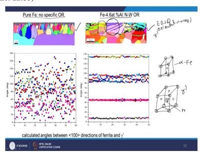
What is shown in this slide (refer to above figure) is on top here these are the again the electron backscatter diffraction orientation maps and for the nitrided iron aluminum alloy and for pure iron. What is the meaning of orientation map here you see that you have all these plate like features are of iron nitride  $\gamma'$  and these other you know the rather homogenous features are the original ferrite grain boundary.
