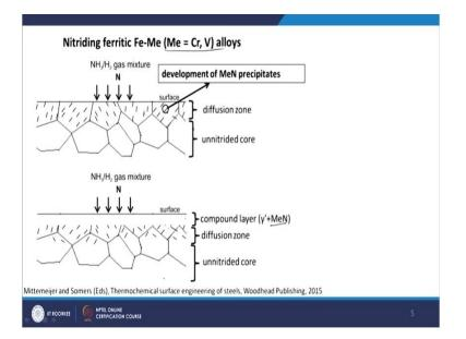
So, now how do we understand this? By here in this slide (refer to above figure) we are showing schematically how the process runs in the case of this easy nitride formers. So, so the nitrogen diffuses inwardly from you know it is supplied from the dissociation of ammonia and this is defuses inwardly and because these nitrides can easily develop you start to form their alloying element nitrides.
