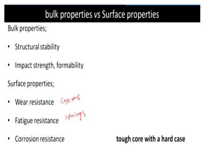
So, we would like to have the gear teethes where you have the loading, so that surfaces of the gear teeth should have highest wear resistance to have a long service life. So, that is one aspect and next is that fatigue resistance. So, for example, a spring and then these springs are under constant variation in the loads they will be operating.
