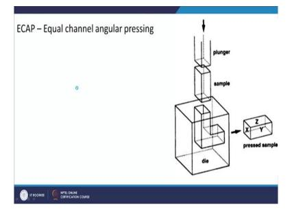
So far, first and very popular or very common process where people want to impose a lot of a strain in the material is called Equals Channel Angular Pressing (ECAP). As you can see, again the idea of not changing the cross-sectional area can be seen here because as the name suggests it is equal channel, so, channel size has to be equal. So, you can see a plunger is here and your sample block is like a cuboid and you have the same size of cavity in the die.
