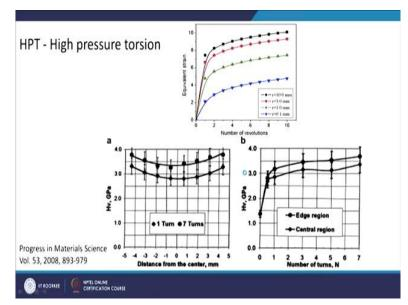
So, you can see numbers of revolutions are shown on the x-axis here, 2 revolutions has gone or 3 revolution for up to 10 they have gone. And they have also plotted what is the equivalent strain which you are putting in the material that is also of course going up and this is at different radius. So, you can understand that when you do a torsion experiment, the strain will increase as a function of radius from the centre, at the farthest point you will have maximum strain.
