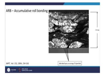
You can see in this micrograph that how accumulated role bonding layers are seen. So, you can see that all these black lines here, these are the interfaces where the stacking was done. So, when you do the stacking there has to there will always a interface will be formed. This is the initial layer and then you are stacking it so, you will also see the effect of the interface. So, all these are interfaces here.
