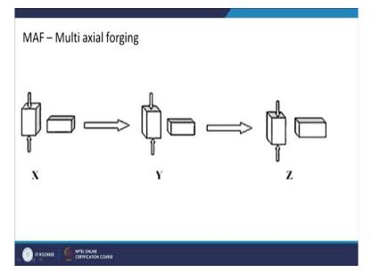
So, basically the idea is that you start with a block like this, which has a higher length in one direction and you forge it. So, what it will do it will flow in this direction when you are forging like this and now you will have a higher length in one of these directions. And it will be because you have a constant volume processes during plastic deformation, volume constancy is there, the reduction in the other two sides will be again the block will look similar to this.
