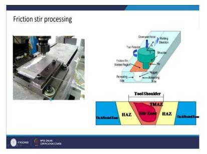
So, as you can see this, these are two sheets. There is a joint here. This is actually right now in a welding condition. So, what you are doing is, you have a tool which is rotating and you are also applying a normal load here, along this direction, and there is a rotation. This shoulder surface if I want to see from this side, if I do not want to see in perspective, it will look something like this, let me change the colour here.
