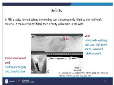
Now what will be the defects which you can encounter during the processing, few defects are shown here (above figure). And people have kind of now worked out that how we can remove these defects. So, one defect which is called void which can occur in the advancing side on the just below the shoulder. So, this is be, usually because of inadequate, you are not able to apply a sufficient normal force to the tool.
