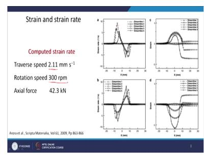
So strain rate if you see here (refer to above figure), the strain rate achieve is around 10 per second. These of the two conditions, I am not sure about the conditions right now. But the rotation speed was taken as 300 rpm and the traverses speed was 2.1 mm per second. So, to just get an idea about strain rate, the strain rate achieved is around 10 per second. And the strain achieved is around 3 in the in the stir zone.
