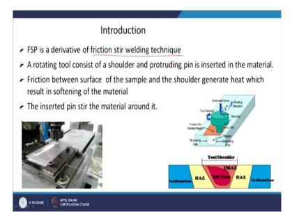
So, looking at the friction stir processing technique, again a very simple technique you can use if you have a milling machine in your lab or in your department you can use it very easily. Basically, you need a vertical milling machine. So, what it has is that you have a tool which contains a shoulder and a pin. So, shoulder is just touching the surface of the work piece with certain normal force.
