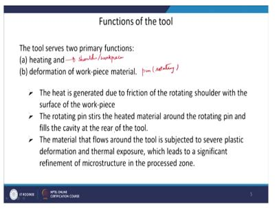
So, function of the tools already we have discussed. So it serves primarily two functions: heating and deformation. So heating is primarily through friction between shoulder and work piece. And deformation is primarily through the rotating pin, shoulder also contribute to some part of the deformation, but primarily it is the pin. So, heat is generated due to friction of the rotating shoulder with the surface of the work piece.
