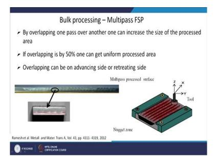
So, basically this is a macrostructure of the same multi pass technique. And in this work the overlapping was done by 50% on the retreating side. You can do overlapping on the advancing side as well as on retreating side. So, you can see that very a big sheet is kind of processed. And if you see in a smaller sheet, effect of individual passes can be seen on the microstructure.
