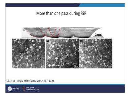
Now, another advantage of FSP is that you can do it by doing multiple passes. I can extend the amount the area of deformation. So, in one pass I can only affect maybe the area around pin size. If my pin size is around lets say 6 mm so, the area affected will be around in that range only 6 mm or so, but if I want to have larger volume or larger area to be processed, what I can do is I can do multiple passes.
