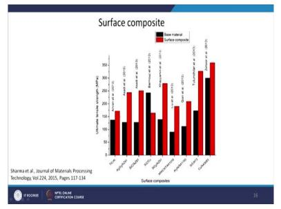
From a review paper, different set of materials, combination of matrix material and the ceramic particle that what kind of strength you will be able to achieve (refer to above figure). So, the black one is showing the base material and the red one is showing you the surface composite. So, there is a very good increase in the strength of the material when you introduce the surface or when you make a surface composite.
