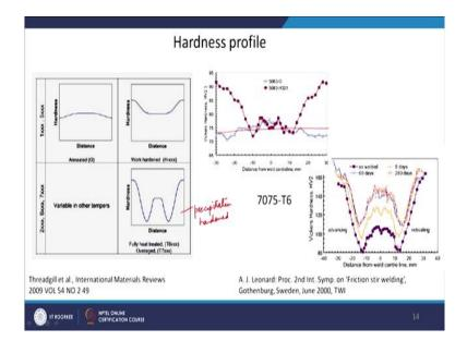
So, if you see in this schematic, there are three conditions are shown for aluminium alloy. Basically, you have annealed condition and in aluminium alloy, there are two different set of alloys, one which are precipitation harden and another which are non-precipitation hardenable. So, in those materials you can have work hardening. So, in precipitation hardenable material if you see the the hardness profile, the profile will be something like this (refer to above figure).
