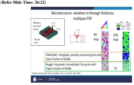
So, suppose this (refer to above figure) is my sheet, this is the thickness of the sheet in which this is your pin and this is my shoulder and which is rotating. So, you can see that only if I see the microstructure will show some basin like this. So, only this part of the microstructure will be affected. The rest of the microstructure in the thickness direction will not be affected that much. So, that is what is characterized here.
