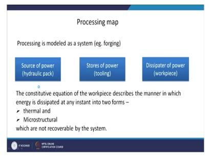
So, already we know how the forging process takes place. You have a hammer or movable ram and your work piece is there and you are having a compressive deformation. So, what is moving the ram? The movement is by power source which is moving that ram and that is the hydraulic system in this case.
