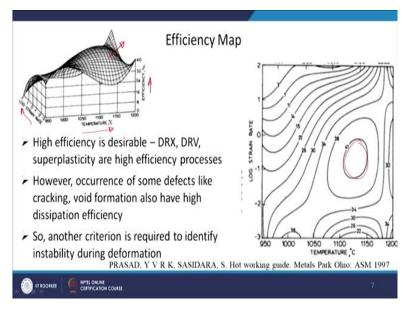
So, you have log strain rate on y-axis, temperature on x-axis and efficiency on the z-axis and there is some three dimensional envelope is there. If I take a section out of it, at any particular efficiency, I should see something like contours (refer to above figure). So, you have contours, which are coming from three dimensional envelope and now it is a two dimensional contours which are giving you the efficiency at different places.
