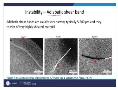
For example, few images are given here. This is an image for adiabatic shear bands (refer to above figure). These are very narrow typically 5 to 500 micron and they consist of very highly sheared material. So, this happen as the name suggests because of adiabatic heating. So, we know that when you are deforming at very high strain rate you can also see the strain rate is mentioned here,  $1 \times 10^3$  and s<sup>-1</sup>  $3 \times 10^3$  s<sup>-1</sup>.
