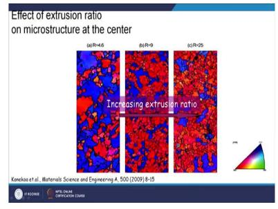
This is the effect of increasing the extrusion ratio that is the ratio between the what is coming out after extrusion and what is you are putting in. And as you can see as the extrusion ratio is increasing because you are putting more strain. The grains are very coarse here big grains are seen. Again only two type of grains one is red one that means 001 axis is coming out or blue one that means 111 axis is coming out.
