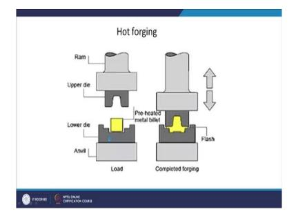
The next process is what we call as hot forging so very simple process basically there are two rams. So, this is a fixed ram then there is a moving ram here and then you kind of bang the material at a very high strain rate. Strain rate you can choose depending upon the rate at which you are hammering the material. So, it is a similar process like a hammer which you must have seen any blacksmith doing next to a road who is working on material or steel that they are hammering the material.
