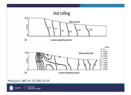
If you see a typical deformation process during hot rolling. So, basically I can say that here I am talking about the strain distribution. So, you can see that x-axis along the rolling direction and y-axes is where you have the thickness of the material and these are some work I have taken from journal called journal of material processing technology. So, basically what they are trying to show here is that; what is the strain distribution at different stages during the rolling.
