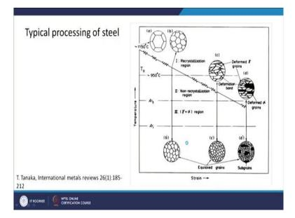
Now this is a typical processing of steel and just to show you that when you do a processing in industry what are the different stages of processing the material has to go through. So, as you can see the deformation or the material is starting somewhere from 1150 degree Celsius and these hatched regions here these are the regions where you have imposed strain in the material. So, as you can see understand that these are all continuous processes.
