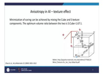
If you see anisotropy in aluminium alloys effect of texture (refer to above figure), minimisation of earing can be achieved by mixing the cube and S texture. These two components if you mix then the earing phenomena is kind of a distributed throughout the you can say circumference and the optimum volume ratio of these two is S and cube is 1.67:1. If you have this kind of mixing of the two texture components then you will be having a good formability.
