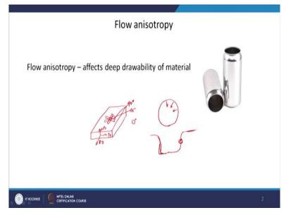
And that is what we have discussed earlier also that when you are deforming or you are doing a deep drawing of any sheet material, there is a flow anisotropy. That means, let us take a material or a roll sheet for example. So, this is my rolling direction, transverse direction and normal direction (refer to above figure). Suppose I am measuring the flow properties in this direction.
