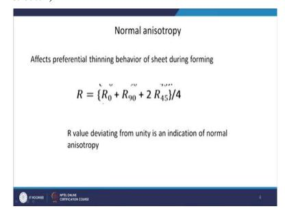
Another value of importance is called normal anisotropy. And that is basically the thinning characteristic of the material.
