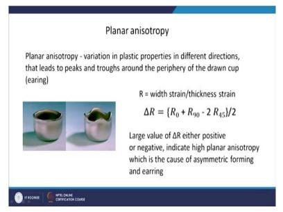
So, this kind of anisotropy develops what we call as earing phenomenon as already have told you. So, in this direction the material is not able to deform but in this direction material is able to deform that is why you are seeing that the material got pulled by the punch whereas in this case it the deformation took place material did not pulled by the punch but other problem will always be there that will be thinning here, it will get thin in this location (refer to above figure).
