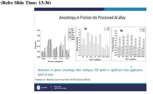
There is another work of our survey where we studied the anisotropy in fiction stir processed aluminium alloy. So, in the first figure, we have different texture components copper, S, Brass, Goss and Cube. And on the Y axis their fraction is noted down. So, basically these (refer to above figure) are the different friction stir processing condition there is one module on severe plastic deformation, there we have discussed the friction stir processing in more details.
