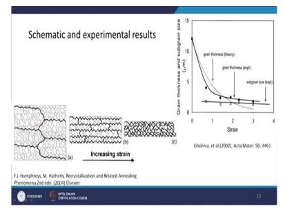
So, this is what is the schematic mechanics. You can see that there are some big grains here (refer to above figure0 and within them there are some small sub grains are formed as you keep deforming. What will happen, these kinds of serrations will form in the high angle grain boundary. And within that you can see the in some cases 1 single sub grain is there in some cases there are 2 sub grains are there and the serration, the wavelength is all most equal to the sub grain size.
