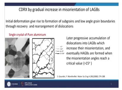
There is some work on the single crystal of pure aluminium was done. And their people have seen that the microstructure initially is getting divided into sub grains and that is slowly converting into high angle grain boundaries. So, a single crystal now is dividing into some low angle grain boundary areas. So, this dotted one is even less than 1°, the lighter ones are 1-6°, slightly darker ones are 6-15° and very bold ones are the 15-30°(refer to above figure).
