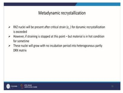
There is another one type of dynamic recrystallization which is called meta dynamic recrystallization a very interesting phenomenon. Basically, it is not a kind of a typical type of dynamic recrystallization it actually happens because suppose a discontinuous dynamic recrystallization is taking place and recrystallized nucleus have already formed at the critical strain.
