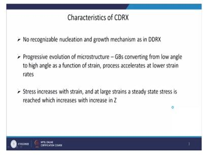
Now, what are the characteristics of continuous dynamic recrystallization, as we have already seen in discontinuous dynamic recrystallization, you have nucleation and growth mechanism whereas, in this case of course there is no nucleation and growth separate as mechanism. In fact, in this you have progressive evolution of microstructure. So, it is a continuous kind of process, where grain boundaries are converting from low angle to high angle.
