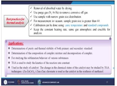
Best practice for thermal analysis, generally removal of absorbed water by drying. Use purge gas like nitrogen or maybe the helium to remove the corrosive off gas. Use sample with narrow grain size distribution. For measurement in vacuum, sample grain size is greater than 60. Calibration can be done using Curie temperature and the standard compounds. Keep the constant heating rate, same gas atmosphere and crucible for analysis.
