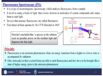
Next technique is called the fluorescence spectroscopy in short generally we are calling it as FS. It is a type of electromagnetic spectroscopy which analyses fluorescence from a sample itself. It involves using a beam of light that excites electron in molecules of certain compounds and causes them to emit light. Devices that measure fluorescence are called flurometers. First, observed from quinine by Sir J.F.W Herschel in 1845.
