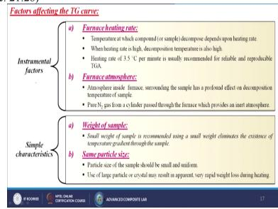
Instrumental factors, what are those? Furnace heating rate: temperature at which compound or maybe the sample decompose, depends upon heating rate. When heating rate is high, decomposition temperature is also high. Heating rate of generally 3-3.5 ° C per minute is usually recommended for reliable and reproducible TGA. Second one is called the furnace atmosphere: Atmosphere inside furnace surrounding the sample has a profound effect on decomposition temperature of sample.
