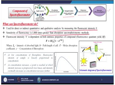
So, generally it is 750, 75-450 watt, high pressure xenon arc lamp or maybe the lasers. Then excitation Monochromator, then sample holder either it may be made by quartz optical glass or maybe the plastic cells. Then emission Monochromator and last we are having the detector or maybe the photomultiplier. What can spectroflurometer do? Used for direct or indirect quantitative and qualitative analysis by measuring the fluorescent intensity F.
