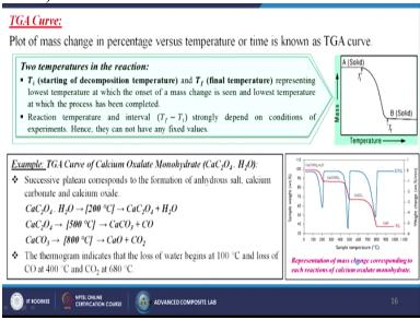
Generally the TGA curve is looks like this. So, plot of mass change in percentage versus temperature of time is known as the TGA curve. So, here in this case we are giving the mass in maybe generally into the weight percent and in this case generally we are giving the temperature in maybe  $^{\circ}$  C. So, two temperatures in the reactions in this particular case T<sub>i</sub> that is the starting of decomposition temperature and T<sub>f</sub> that is the final temperature.
