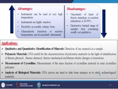
Then what are the advantages? Instruments can be used at very high temperatures. Instruments are highly sensitive. Flexibility in crucible volume or maybe the form, characteristic transition or reaction temperatures can be accurately determined. Of course there are certain disadvantages
