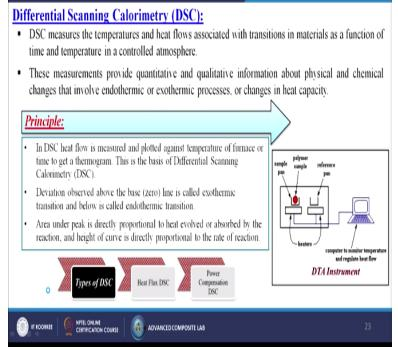
Next one is called the differential scanning calorimetry or maybe the DSC. So, DSC measures the temperatures and heat flows associated with transitions in materials as a function of time and temperature in a controlled atmosphere. These measurements provide quantitative and qualitative information about physical and chemical changes that involve endothermic or maybe the exothermic process or change in heat capacity.
