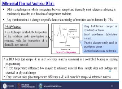
Then next one is called the differential thermal analysis or maybe the DTA. So, DTA is a technique in which temperature between sample and thermally inert reference substance is
