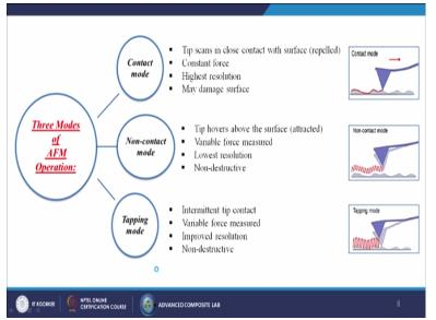
Generally there are three modes of AFM operations. First one is called contact mode in which the probe is touching the surface of the materials. Tips scans can close contact with surface repelled. Constant force, highest resolution, may damage the surface. Second one is called the non contact mode, tip hovers above the surface attracted, variable force measured, lowest resolution, non destructive.
