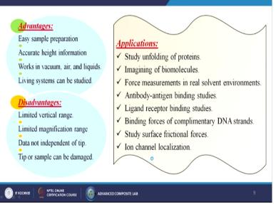
What are the advantages? Easy sample preparations, accurate height information, works in vacuum, air, and liquids, living systems can be studied. What are the disadvantages? Limited vertical range, limited magnification range, data not independent of tip, and tip or sample can be damaged. Of course there are certain applications, what are those?
