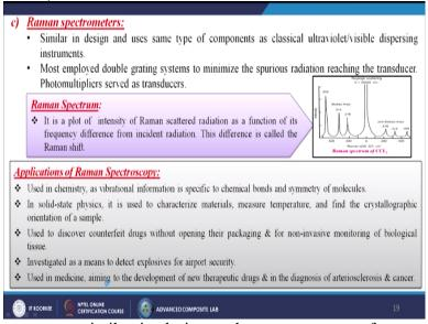
Then Raman spectrometers: similar in design and use same type of components as classical ultraviolet or maybe visible dispersing instruments. Most employed double grating systems to minimize the spurious radiation reaching the transducer photomultipliers served as transducers,
