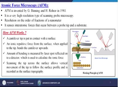
AFM is invented by G. Binning and H. Rohrer in the year of 1981. It is a very high resolution type scanning probe microscopy, resolution on the order of fractions of a nanometer. It senses interatomic forces that occur between a probe tip and a substrate. How AFM works? A cantililever tip is put in contact with a surface itself, a cantilever tip here it is touching the surface.
