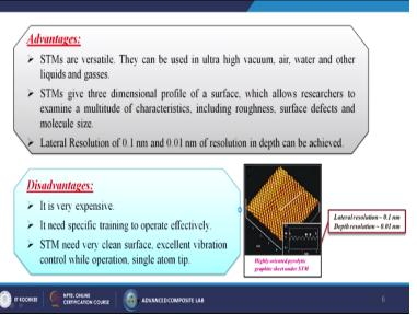
What are the advantages? STMs are versatile. They can be used in ultra high vacuum, air, water and other liquids and gasses. STMs give three dimensional profile of a surface, which allows researchers to examine a multitude of characteristics, including roughness, surface defects and molecule size. Lateral resolution of 0.1 nm and 0.01 nm of resolution in depth can be achieved. Of course there are certain disadvantages; it is very expensive, it needs specific training to operate effectively.
