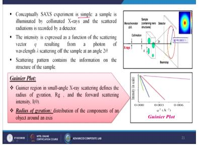
A sample is illuminated by collimated x-rays and the scattered radiation is recorded by a detector itself. so the collimations, so monochromated x-rays is going, this is the sample containing nano structures and then we are having the detectors and it looks like this, the intensity is expressed as a function of the scattering vector q resulting from a photon of wavelength lambda scattering of the sample at an angle 2 theta.
