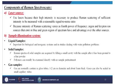
Use lasers because their high intensity is necessary to produce Raman scattering of sufficient intensity to be measured with a reasonable signal-to-noise ratio. Because intensity of Raman scattering varies as fourth power of frequency, argon and krypton ion source that emit in blue and green region of spectrum have an advantage over the other sources.
