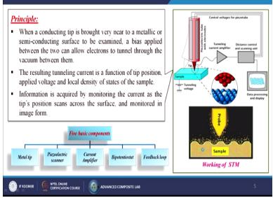
What is the working principle? When a conducting tip is brought very near to a metallic or semiconducting surface to be examined, a bias applied between the two can allow electrons to tunnel through the vacuum between them so this is talking place. The resulting tunneling current is the function of tip position, applied voltage and local density of state of the sample itself.
