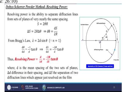
Now what we are getting from the Debye-Scherrer Powder Methods Resolving power, if you are going to calculate the resolving power, so resolving power is the ability to separate the diffractions lines from sets of planes of very nearly the same spacing, so here in this particular case what we are going to do we are putting the incident beam and then it is falling on to the samples and the reflected beam is falling on to the film in this particular point.
