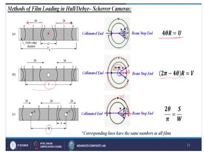
Now there are so many methods of film loading on the Hull Debye-Scherrer Cameras so first when we are talking about these say suppose we are having that here the  $\theta$  is equal to 0 degree here the  $\theta$  is 90 degree, two  $\theta$  is increasing in this way, two  $\theta$  is increasing in this way from 0 both the sides so this is known as the knife-edge shadow, so these distances is known as the capital U.
