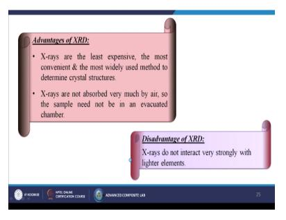
So now we are going to discussed about the advantage of the XRD, so X-rays are the least expensive, the most convenient & the most widely used method to determine the crystal structure X-ray are not absorbed very much by air, so the sample need not be in a evacuated chamber, but of course there are been certain disadvantages also so X-ray do not interact very strongly with lighter elements.
