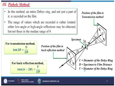
So now we are going to discussed about the Pinhole methods so in this methods, an entire Debye ring and not just a part of it, is recorded on the film, the ranges of values which are recorded is rather limited either low-angle or high angle reflections may be obtained but those in the median range of theta so in this particular case we are putting one spacing over here, and now some rays maybe it has transmitted through samples or may be it has been reflected through samples.
