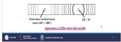
Now how it looks, Powder Diffractions Films the cones of diffracted radiations intersect the cylindrical strip of film in lines or arcs and when the strip is unrolled and laid out flat, so after that we are making the film in a flat and we are getting the lines in such a manner some lines are strip some lines are in a circular shape, or may be the round shapes, so each diffractions lines is made up of a large number of small spots each from a separate crystal particle the spots lying.
