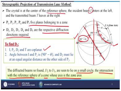
So in the next slides we are going to discuss about the stereographic projections of transmission Laue methods, so the crystal is at the center of the references sphere the incident beam is I, so this is the I enters at the left, so this is the left side and the transmitted beam T leaves at the right side, now this P1, P2, P3, P4, P5 this five planes belonging to a Zone, so this is known as the zone D1,D2,D3,D4,and D5 are the respective diffractions directions required.
