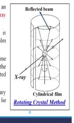
Now we are going to discussed about the second types which is nothing but the known as the Rotating crystal method, so in the rotating crystal methods a single crystal is mounted on an axis normal to a monochromatic X-ray beam, so in this particular case we are putting the crystal in this particular positions a cylindrical film is placed around it and the crystal is rotated about the chosen directions, the axis of the film coinciding with the axis of rotations of the crystal also.
