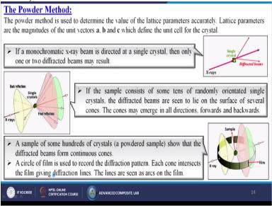
So how we are going to do the powder method, the powder is used to determine the value of the lattice parameters accurately, lattices parameters are the magnitude of the unit vectors A.B and C
