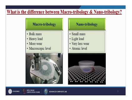
So, what is the difference between macro Tribology and Nano Tribology? In the macro Tribology it is the bulk mass, the size and weight of that particular equipment or may be the machines are bigger, heavy load generally you were applying heavy load on to those machines or maybe they are generating heavy power or maybe heavy energy or maybe heavy load. More wear maybe there are n number of materials is touching together.
