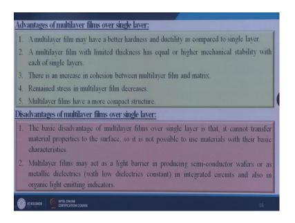
So when you are talking about the advantages; a multi layer flame may have a better hardness and ductility as compared to single layer. A multi layer flam with limited thickness has equal or higher mechanical capability stability with each of single layers. There is an increase in cohesion between the multilayer film and matrix, remained stress in multilayer film decreases; multilayer films have a more compact structure. So, these
