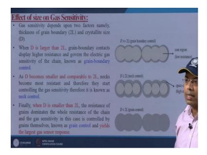
So, gas sensitivity depends upon two factors namely the thickness of the grain boundary that is known as the 2L and the crystallized size which is known as the capital D. So, in this particular figure I am trying to explain that how these different sizes are actually affecting the gas sensing technology.
