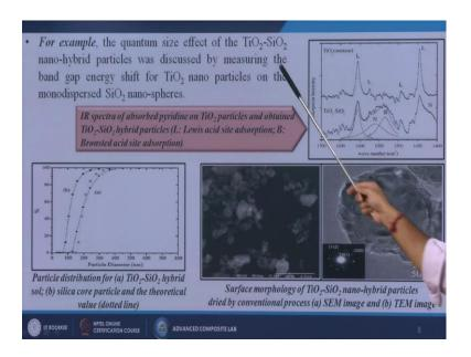
Next that is also an example, so here the example is that quantum side effect of titanium dioxide, silicon dioxide nano hybrid particles was discussed by measuring the band gap energy shift for titanium dioner particles on the monodispersed silicon dioxide nano spheres. So, here actually the material is the hybrid composites initially we have taken
