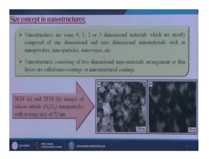
So, nano structures are some 0, 1, 2 or 3 dimensional materials which are mostly composed of 1 dimensional and 0 dimension nano materials such as nanopowders, nanoparticles, nano-wears. So when we are talking about any nano particles, the nomenclature
