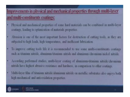
First one is called the physical and mechanical properties of some hard materials can be combined in multi layer coatings leading to optimization of material properties. Yes of course, that actually totally depend upon our requirement, I can put some kind of soft materials on top of that I can put some kind of hard materials, again top of that I can put some kind of soft materials, it totally depends upon our requirement.
