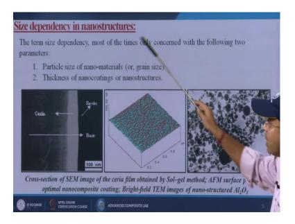
Already I have told you that term size dependency most of the times only concerned with the following two parameters, one is the particle size of the nano materials or maybe the grain size or maybe the crystallites site and the second one is that thickness of nano coatings or the nano structures; that is how much layer may be a single layer, may be a multiple layer; I am trying to put onto my substrate or may be that onto our materials.
