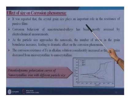
So, in that some literature it was reported that crystal grain size plays an important role in the resistance or passive films; that means, corrosion behavior of nano structured alloys has been mostly assessed by the electrochemical measurement, as the particle size approaches the nano scale, the number of atoms in the grain boundaries increases leading to dramatic effect on the corrosion phenomena, so this is the basic principle of this particular slide.
