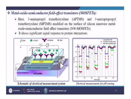
So, 3-aminopropyl trimethoxysilane and 3-mercaptopyl trimethoxyssilane MPTMS, these all are the two materials by which we can modify our nanoparticles. So, from the right hand side figure you can understand that the green color is giving the unmodified nanoparticles and then metal oxides nanowire metal oxides and then right color is giving the modified it by the APTMS and the blue color it is giving with the modified by MPTMS.
