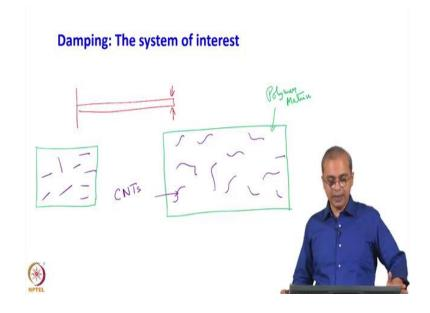
So, what is our system of interest, our system of interest is basically a composite material in which we have added carbon nanotubes? So composite materials, in this case, a polymer-based composite; so, the polymer itself will have some damping properties. So, if you just have the plain polymer and you put some vibration into it, you can see how the vibration damped, is getting damped.
