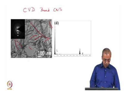
Similarly, if we do the CVD synthesis and we look at the CVD based CNT. So, this is CVD based CNTs, clearly, you can see lot of wrinkling and coiling and so on. So, plenty of movement of that nature you can see almost everything is coiled, you can see here this is curved, you can see these are all curved you can almost everywhere you can see a curve, you can see curves here, curves here, I am just highlighting a few.
