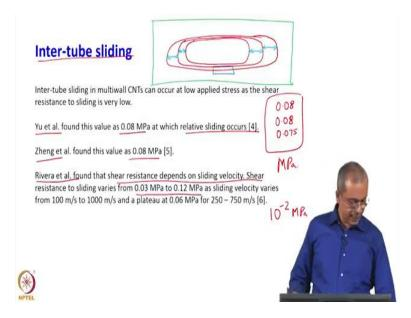
There is another way in which CNTs can do damping and that is called inter tube sliding. So, now, in this case, what we are saying is, if you have the nanotube and I now draw it in a bit more enlarged way for a specific reason; we have a nanotube here and again it is in some matrix, it is in some matrix.
