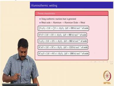
Ok so the reaction what you see over here is the exothermic reaction of reduction of iron oxide metal oxide by aluminum.
