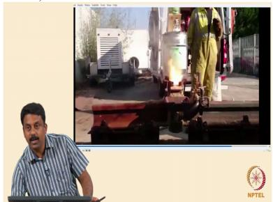
started pouring down from the bottom cavity towards the mould and these are all runners and risers on the side. So now it is done.
