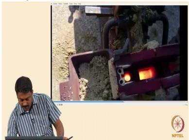
You see that inside. So that is the weld cavity. So this is the mould and inside you will have the weld cavity.
