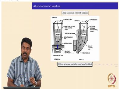
would actually work based on the principle that the moment the temperature goes above certain temperature it will crack and then liquid metal would start filling the weld cavity, yes. Is it clear?
