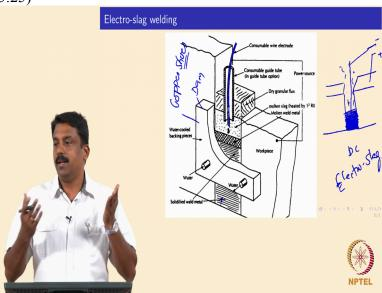
So first is electro-slag welding. Okay. The electro-slag welding is widely used for thicker sections. So we process work like this. Okay. So we have filler material. Is not it? So this is the wire, filler. Right? And filler is actually first fed into the weld cavity. So this is the interface to be
