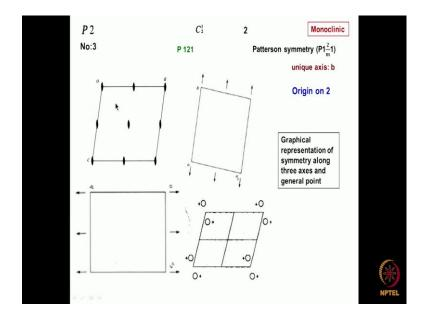
Then next what is the information which is being given is essentially the unit cell and this is the unit cell 1 projection and in this projection the what are the symmetry elements this is for a P 2 means that only 1 2 fold rotation is there and the detail symbol if you look at it P 2 is 121. That means that along x axis 1 fold rotation, 2 fold is along the y axis and 1 fold along the z axis.
