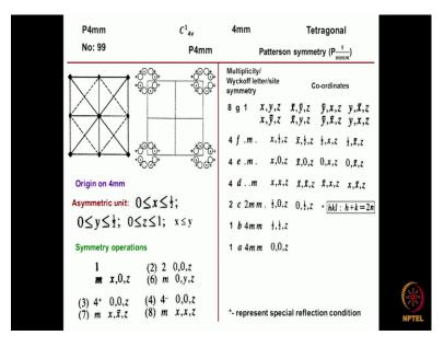
Now, let us look at a P4mm, here it is a 4 fold symmetry, 2 mirrors are also associated with it, the way in which it is represented is that these are all the positions of a 4 fold symmetry lattice points then here we have 2 fold then mirrors which are there the motifs, these are all points if we keep your motive at this particular point it is lying on a mirror. So, it is called a special position if you put it here it has a symmetry which is 2mm. So,
