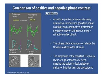
So, now we will see the some of the other aspect of this phase plate; comparison of positive and negative phase contrasts systems. So, you have this positive phase contrast plate and this is a negative phase contrast plate. So, they do exactly the opposite actions in order to produce a different, different contrast effects as you can see in the images.
