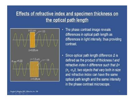
Let us now look at the effect of refractive index and the specimen thickness on the optical path length. We have already seen that what is optical path length, and which is having a significant role in this phase contrast microscopy. Let us see what it is.
