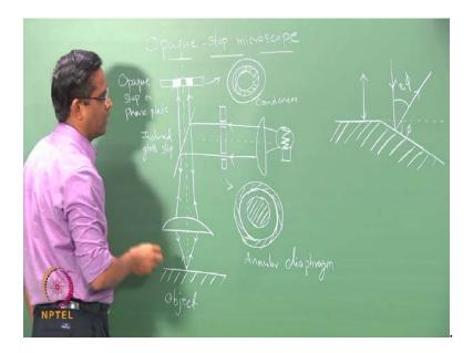
So, let me draw this schematic of the opaque stop microscopy. So, we will have the light source here and then you have the condenser. Like we have drawn yesterday, it is a glass slip, which is inclined at 45 degree then you have this is objective and then you have the object. So, light rays are first coming through this objective and then going back like this. Then it is suppose to go to the eyepiece like this. So, this is inclined glass slip.
