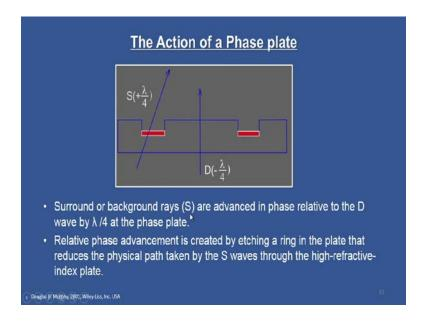
So, let us look at the action of a phase plate. So, this is a phase plate, a typical phase plate will have. And you see that light rays are passing through this; one is advanced, one this annulus ring is advancing the S ray by plus lambda by 4; and the other region of the phase plate is retarding the wave by lambda by 4.
