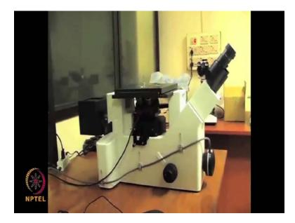
Now, what I am going to do is I am just going to introduce you to the some of the microscopes. What is coming on the screen is a typical a metallurgical microscope. There are two basic types of microscopes; one is vertical type, another one is inverted type. So what you are now seeing is inverted optical microscope. I will just show some of the main parts which we have talked about.
