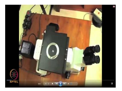
This is the specimen stage. Since your vertical microscope, this is the specimen stage will be on the top.
