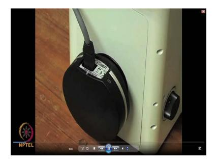
And this is a CCD camera which is being attached to this microscope.
