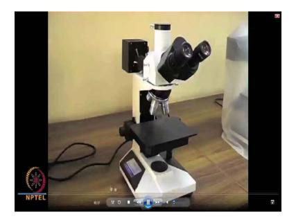
And what now you are seeing is another vertical simple type microscope, a standard microscope. In any of the metallurgical laboratory you see that oculars.
