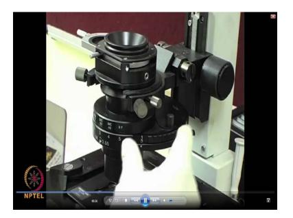
So, I will just describe these microscopic parts so that you will get familiar with what are the important things you need to understand. What is that being shown here it is a polarizer; and you when you do not use that polarizing mode, then it will be a slot for a bright field mode. Then you also have a kind of a condenser aperture lenses in this which is having a different slots. I will talk about it in much more elaborately in the next class.
