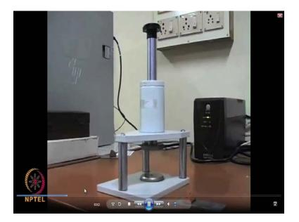
So, this is the tool which is called Leveling Press to make the solid specimen in a same level, using this plasticizer.
