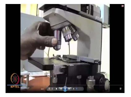
Or it is having an interface with that computer you can clearly see that the objective lens is now as I mentioned. You are also observing that you know some of the letters are written on the objective which they talk about the magnification some refractive index and whether it is oil or a dry all those information are given on this objectives. Usually it is comes with 5 x, 10 x, 20 x, and 40 x, and then sometimes 50 x and it goes up to 100 x also depending upon the microscopic system.
