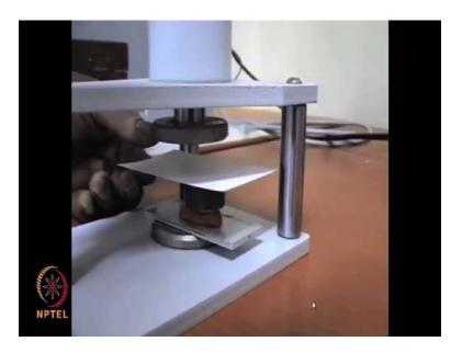
And this is how the solid metal pieces leveled using this a leveling press, and then it will be placed on this microscope as you can see that. I will get into the details of all this preparations in a separate class.
