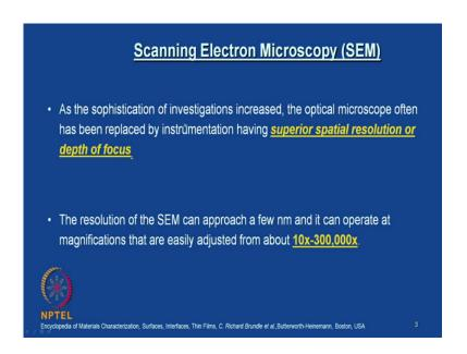
As the sophistication of the investigation increased, the optical microscope often has been replaced by instrumentation having superior spatial resolution or depth of focus. The resolution of the SEM can approach a few nanometers, as I mentioned and it can operate at magnifications that are easily adjusts from about 10x to 300,000x. Of course, this can be a subject of instrumentation we will talk about it in appropriate time.
