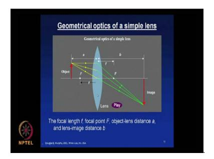
So, now let us look at the geometrical optics of a simple lens. You have the glass lens and this is in object which you have here red in color and then, the light is passing through the lens and then, it get focused on the other end where the image is formed and that the distance between the center of the lens and these two points front there are two points in front of the lens. One is in the front and one is at the back.
