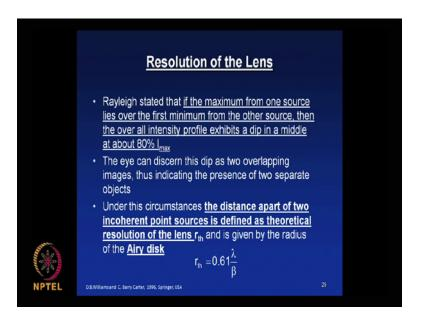
So, Rayleigh stated that if the maximum from one source lies over the first minimum from the other source, then the overall intensity profile exhibits a dip in middle at about
