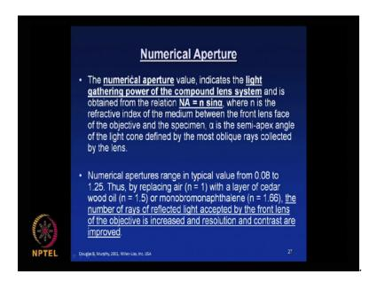
The numerical aperture value indicates the light gathering power of the compound lens system and it is obtained from the relation numerical aperture equals n sine alpha, where n is the refractive index of the medium between the front lens face of the objective and the specimen alpha is the semi-apex angle of the light cone defined by the most oblique rays collected by the lens.
