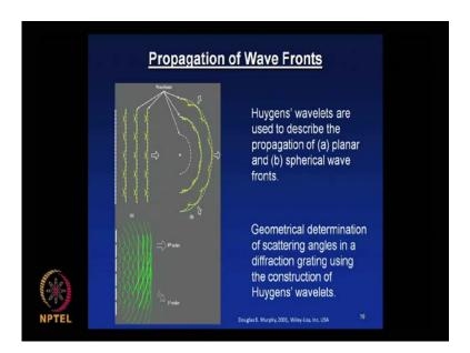
We will see much more detailed information about the diffraction as we go along. If you look at this, how the wave propagates there is a schematic you can see that this is described by Huygens wavelets are used to describe the propagation of a planar and
