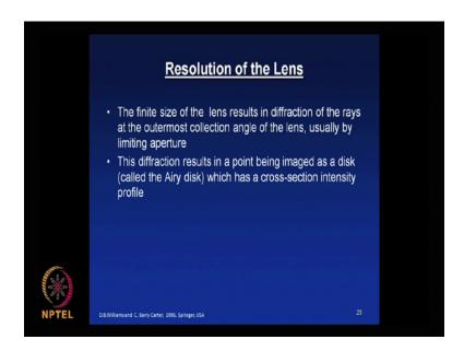
So, the finite size of the lens results in diffraction of the rays at the outermost collection angle of the lens, usually by the limiting aperture. This diffraction results in a point being imaged as a disk which has the cross-section intensity profile.
