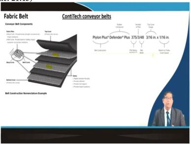
Then you can see here that the fabric belt in a fabric belt there are layers of this fabric they are having this horizontal member and the that is the longitudinal member the transverse member which is called your weft and there is a longitudinal member called your warp they are made together at just like your clothes and then there are a number of them as a layered form. And then we can see over there they say your this layer.
