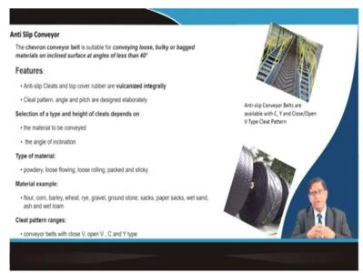
And as I said that in the anti slip conveyor belt number of belt manufacturers they are giving C, Y and V type of the surface roughening and with that they give this glitch on the conveyor belt which exactly serve your purpose so that you can maintain the productivity because if there is a slip of the things materials flow rate will get reduced. So that is why there you will have to be careful about selecting the belt from.
