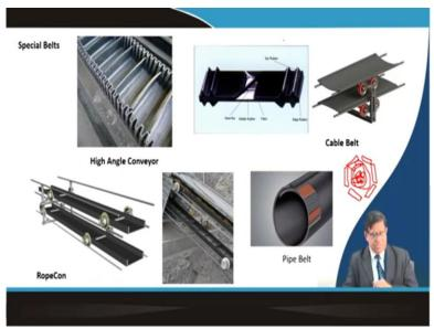
So, we have also some of the special belts in the mining or bulk material handling in plants particularly this high angle conveyor, cable belt, RopeCon, and pipe belt which we have talked about earlier. Now they are the beams that are how this type of special belts will have to be manufactured. So, these are the belt with that your sidewall you can see that this corrugated sidewalls are given and then getting that thing with the flexibility.
