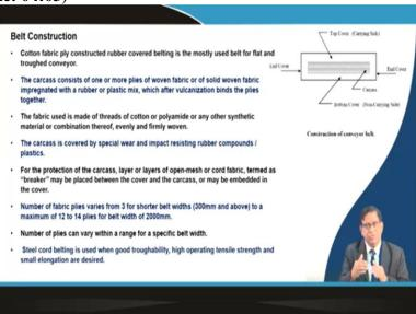
Now as we say that the belt constructions in the figure you can see there is a central part which is the main we say it as a carcass this carcass is the to proper strength of the belt will be coming from how structure of this carcass is made and then it has got a top cover and the bottom cover and covers. Now these covers are that which is exactly protecting the carcass and making this belt usable for different purposes are very important.
