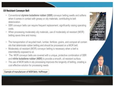
As an oil resistant conveyor belt it comes in different industry it becomes required particularly this when we talk about this SBR rubber material that is your styrene butadiene rubber if particular specific rubber it swells when it is a coming in contact with grease and oily material. So that which will be leading to a belt damage. So that is why such type of rubber are not used in some specific so where you need to handle some of this debrises and all coming from a plant.
