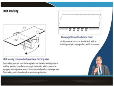
So, the belt tracking is a very, very important area and there such types of self aligning idlers are used for doing so that if the belt goes this way and it will be put into the proper form. So that sometimes if you are giving some adhesive roller into the carrying roller they also help in keeping the belt running true.
