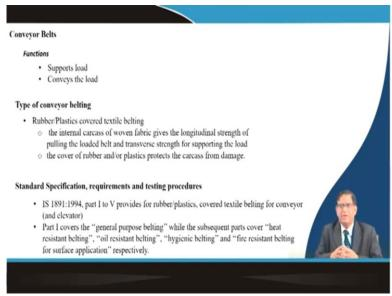
So, as you know that is a conveyor belt what are its main functions? It is exactly it will have to support the load and then convey the load and while that it will also have to for movement whatever the power required that will have to be also taken on it that is it is also working as a that is for the driving the conveyor belt it will be working as a part of this friction drive. So, it will have to transfer the power from the pulley to the belt for its motion.
