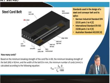
Because selection of the conveyor belt and then replacement of that it will be necessary but in the other type of belt say for example in the mines where your heavy material will have to be carried out the fabric belt they may not be with standing the necessary strength for that exactly. So that is why that steel cord belts are used now in the steel cord belt you can see here that we are having a longitudinal member is steel wire rope.
