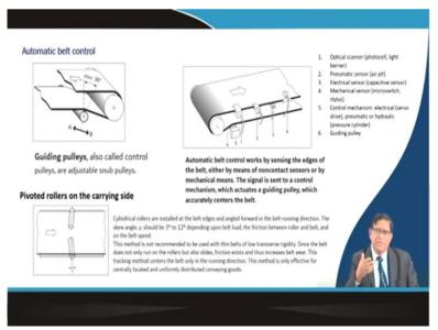
And today the modern machine instruments have come for automatic rib detector that is you can you can for controlling the belt you can have a different type of arrangement like your you can have a guiding pulley one pulley can be kept that will be guiding over there then these different type of sensors they are put together. And then if there is a; that this guiding pulley which is there as an adjustable snub pulley by proper control of that you can make the belt to run true.
