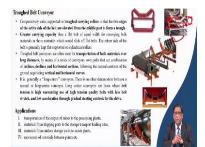
So anyway, coming to this trough belt conveyor, it is exactly compared to the flat belt conveyor, their belts are wider. And then these 2 edges are lifted. So that it will have to make it tough. To forming the trough on the idler you will have to see but one thing is true when the belt is running at that 2 end you have got the belt will be running over this 2 while it is going like this at this stage and at this stage these 2 ends will be flat.
