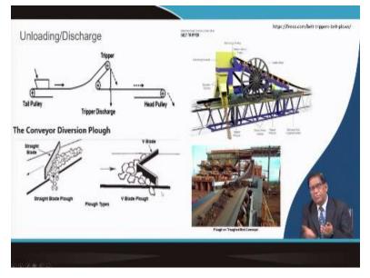
Then similarly in the unloading, I have told you that tripper arrangement, you can see here, there are some wheels and then a rail is there and that is a motor is there. Now, this is just like a trolley it can move towards that means this portion is raised you can see that this conveyor belt, it is coming over here and then it is raised and from there it is going down and then it is going like
