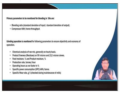
So, you can serve different industry if you know the basic understanding of the system and how it works. Now there is a primary parameters to be monitored in a blending in a silo I in the previous class I was telling you about an example of a silo. Now that in that silo how exactly the blending takes place you will have to measure and what you will be monitoring you will be knowing what is the blending ratio and then how much exactly the thorough put it is coming.
