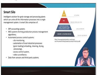
So, we had been telling about this silos which are using there how exactly the total system is done your intelligent solution for the grain storage and processing plants which can unite all the information processes into a single management system and that is a smart silo which comprises of your you will be having a ERP which will be having its accounting system you will be having a manufacturing execution system.
