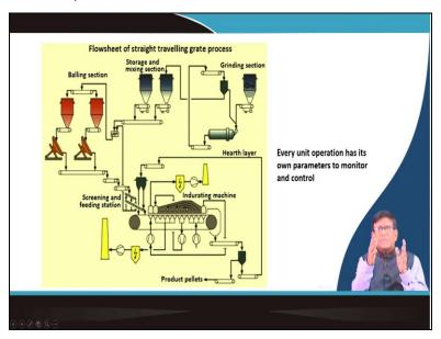
So, this type of things happens in pelleting if this is a pelleting plant you can see over here there are these are the pelletizer in which this is your; in the bowling sections they will make the balls out of it this is a this is having a that eccentric shaft it will be giving a gyration motion and then during that motion this pellet as a green pellet will be coming and then there will be going this is your the grate on which that is exactly the burners for your furnace oil is burned.
