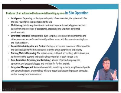
So, features of an automated bulk material handling system the silo operations you will have to have that the intelligence you will have to do some multitasking different operations you will have to have a error free functions you will have to correct vehicle allocation and control that how the materials are coming and taking back then your tracking material balancing then your data acquisition processing and archiving and integrated management can be brought.
