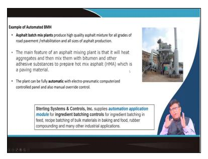
So, these are the area somewhere where you will have to use your automation in the industry. Now for example one that is your the that your when your hot mix has felt when you are preparing the hot mix asphalt in an asphalt plant that is your you are making it a batch mix one big batch is coming and then it is next is coming. So, in a big construction sites they can have a plant like this.
