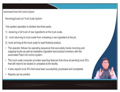
So, this automated feed mill control system that is your receiving load out of the truck scale system that how much material has come how exactly you will be paying for your material which you have done for that you will have to have an automated receiving section. So, that is you might have seen sometimes this trucks are coming and then there is a way bridge on the way bridge it is coming and going there automatically.
