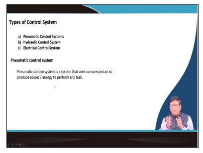
So, this control when you will be actuating exactly the operating the machine there you can have a pneumatic control system, hydraulic control system or electric control system or electro hydraulic electropneumatic and the combination of it.
