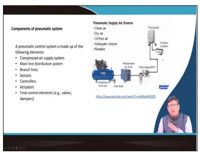
In a pneumatic control system basically you will be having a compressor from that compressor this your air will be that main component will be from the air you are compressing it over there then the it will be going to a pulse to the name this different distribution pattern then there will be it is going to the different branches where you want to give it sensors then it will be having controller it will have actuator it will have the final control system.
