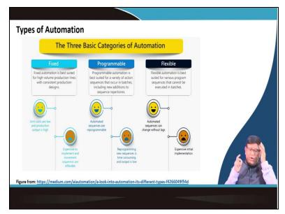
Now, these automations how it could be there, there are different type of degree of automation depending on the work where you are going for doing this automation. Now there is a something called your fixed automation which is exactly wherever there is a high production lines with a consistent production design there we can go a fixed type of where their unit costs are low and the production output is high.
