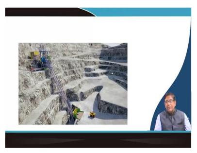
Now, where it could be applied even in some surface mines also, instead of making your truck to move all the around that is ramp and all that thing they go over here. If your material is to be taken over here and from there you are taking that a rail or by conveyor you can take up from that bottom. You can load into that skip that skip can go up over here then give a overturn and then it will do.
