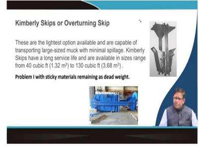
So, this type of devices were designed from the very primitive one it came. Say first Kimberley, a mines name only under that they have, they got an overturning skip. So, this keep is nothing but it has got a that you can see this side rails and then this one here this that you can see a modern F. L. Smith, this overturning skip over here now they have made an arrangement that the material will be loaded over here.
