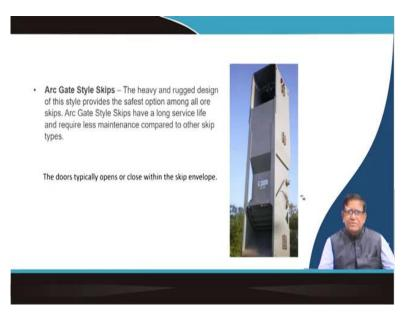
So, similarly, you have got some arc gate. Here exactly you have got the the door which will be a opening and closing by an arc. So, this type of skips are called arc gate type of skips. So, you can see over here how things get innovated. That concept was there that there will be a container which will be loaded by material in underground and it will be brought now. You can imagine now that whether you can make a tabletop model if you are putting it there.
