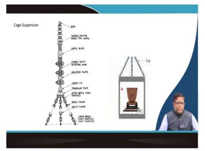
So, here this cage within the cage you will have to have the mine car and then will have to suspend it and then it will have to be lifted. So, there is a wire rope the steel wire rope which is in the rope haulage and all also so, this wire rope will have to be connecting to this cage and these are the suspension chains. This suspension chains, they will be having a shackle on which this cage will be suspended.
