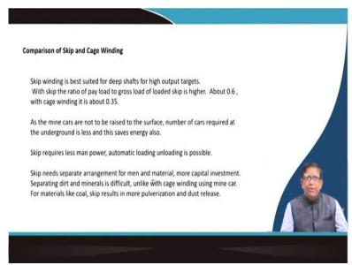
Now, you can think of when you compare this, skip winding and cage winding. So, as I said, the skip winding is best suited for deep shafts for high output targets which skip the ratio of the pay load to gross load of loaded skip is higher that ratio. It can go up to 0.6 in cage of your skip winding but in cage winding your that it goes up to 0.35. Because your that mine car it has get its own weight.
