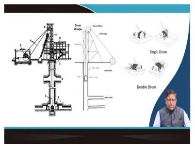
Now that suspended cage is can be brought within the shaft. You can see here in this diagram that your cage is suspended with this wire rope which is coming to your this bunk level, where there will be the cage. From the cage the your mine car will be taken out for dumping the material for the next transportation. And then there is a level to which there will be the safety hook and other safety appliances will be placed.
