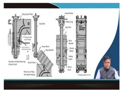
Now, this overturning skip there could be how you can see over here. There is a in the skip, a guide roller, a skip roll is there and then this bucket. Now, you can see by the side of it we have got this dumb roller arrangements. When it is coming to the top it will be brought over here and then, when it comes to the dumping point at that your skip roll plate here it get move and that whole meter become your upside down from this trinion point is here.
