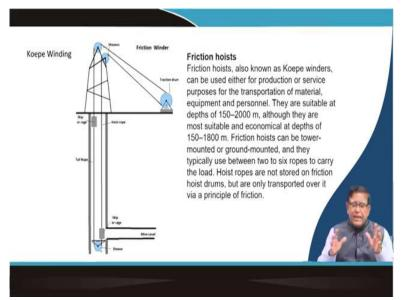
So, these are the things exactly you should keep it in mind. And that winding I have said that by a drum winder, instead of this, what can be done? In the drum you can see here that lot of winding of this your wire rope is here. So that they are wound and unwound and always you are keeping some rope over here. But there is another system in which you can see that this rope is continuously going and below it is returning over here.
