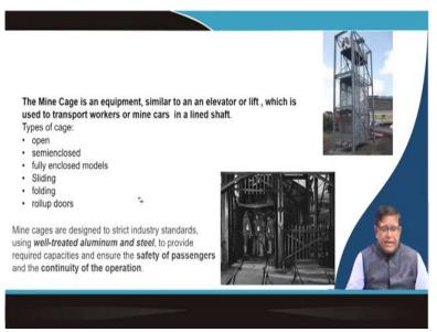
So that means your this you can see here that my cage, this figure which you have seen over here, this is a cage and that cage it can be number of decks. So, this is a triple deck that your double deck cage over here. So that you can just below this another layer the people can be in both sometimes in one layer you can have the person standing another the car standing and the whole thing will be lifted.
