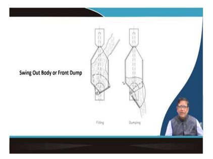
There is this your swing out bodies you can see here this is a skip bucket. Now, in the skip you can see when at the loading station in underground the material is brought inside this by means of a chute. Then, when the material is coming you are keeping your this sector gate of the skip is kept closed. Now, when they will be coming to the up at the your dumping position at that time, your this gate it will swing for opening.
